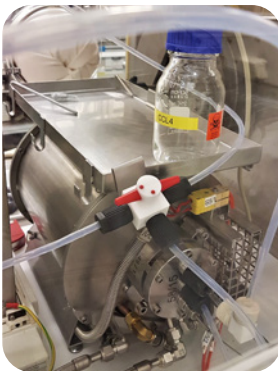
Chlorination reactor (credit: JRC)
